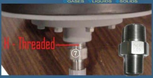
Test heads come as the original "H" (threaded ) 🕜 spud configuration or "G" style configuration (8). "G" Style allows you to swap thread sizes quickly.
