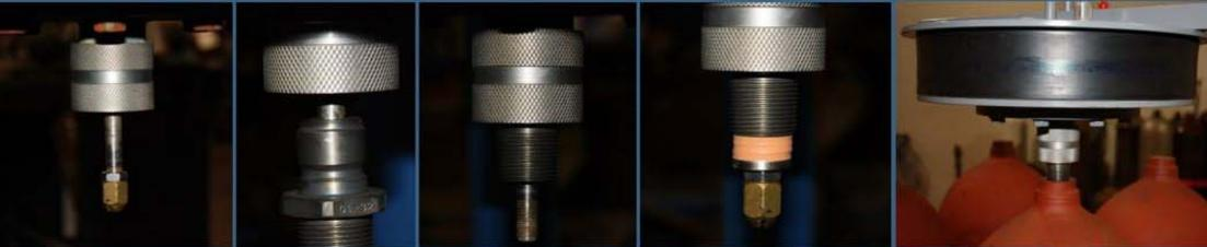
This "G" style uses a quick-connect spud that allows you to change the cylinder side thread in as little as 20 seconds. With the "G" style you have a direct connection to the cylinder rather than using an adapter. This minimizes leak points and wear you would normally see when adapting a spud to fit different cylinder neck threads.
