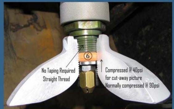
Seals the cylinder test connection with speed seals at the cylinder threads when Low Pressure Hose is applied
