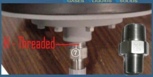
Test heads come as the original "H" (threaded ) 🕜 spud configuration or "G" style configuration (8). "G" Style allows you to swap thread sizes quickly.
