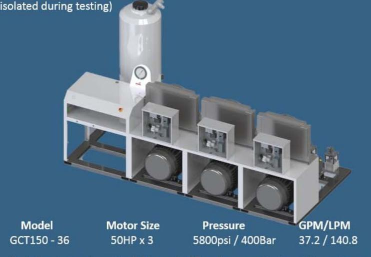
Cycle frequency is controllable up to 15 cycles per minute within system pressure. Cycle results are documented in chart form showing pressure verses time by cycle number. The Cycle Test System incorporates PLC and computer technology to provide fast, accurate, reliable cylinder cycle testing. The flexible platform with PLC controls accommodates a variety of system component options.
