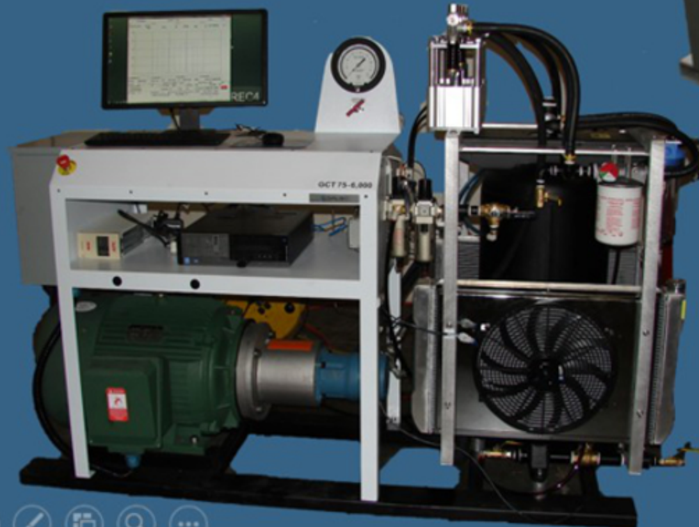
GCT75-6k Pressure:6,000psi Flow: 17.2gpm Medium: Oil
