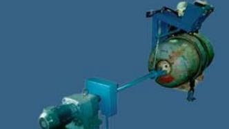
M103-627-334 HORIZONTAL VALVING MACHINE for PRESSURE DRUMS with diameter up to 1000 mm.
