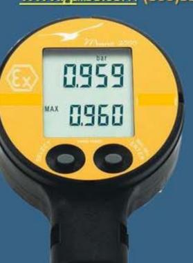
The pressure is measured twice per second and displayed. The top display indicates the actual pressure, the bottom display shows the MAX.- or MIN- pressure since the last RESET.
