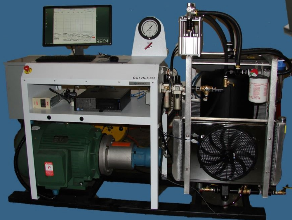
GCT75-6k Pressure:6,000psi Flow: 17.2gpm Medium: Oil
