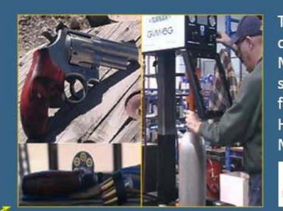
The GVM Safety Shield P/N 14-41-0660 is a bolt on accessory for the GVM-16 valving machine. Made from bullet resistant Lexgard Lexan, the safety shields bullet resistant properties have been field tested by our Quality Assurance Team. The High Impact Safety Shield was able to contain a .44 Magnum projectile from the distance of 10 Feet.
