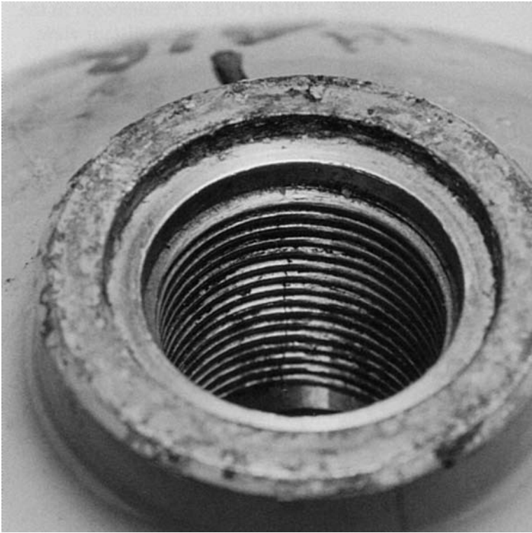
PHOTO 9. A crack easily seen with the naked eye, near the top or O-ring gland. A quick cleaning should be done, enough to verify that it is a crack.
