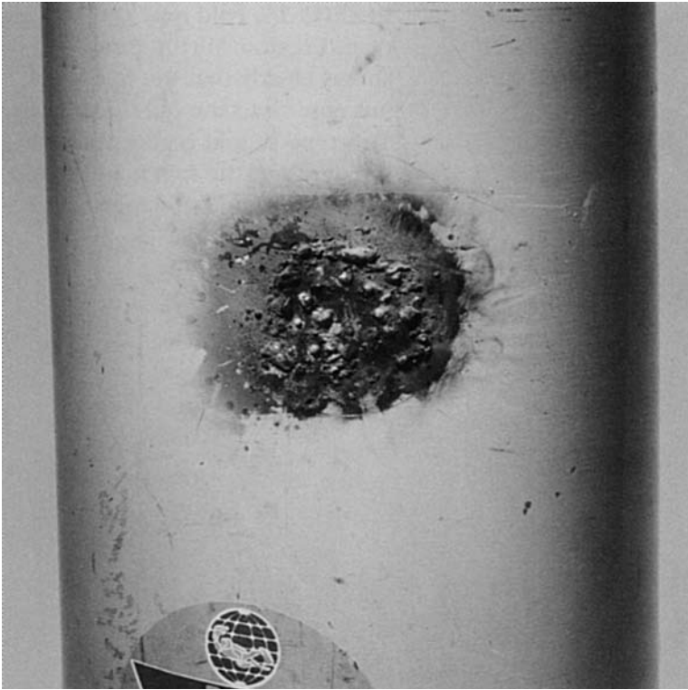
PHOTO 14. Appearance of fire or welding damage done to a cylinder.
