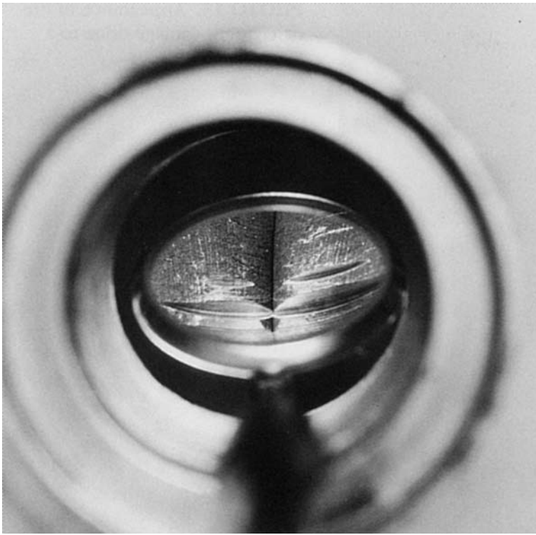
PHOTO 15. Fold near the thread region. Mirror view shows clearly that the fold does not enter into the full-thread area. This type of fold is acceptable if the depth of the fold is estimated to be less than 0.060 inch (1.53 mm).
