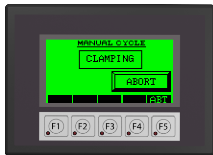
Figure 4-13, Manual Cycle Clamping in Progress
