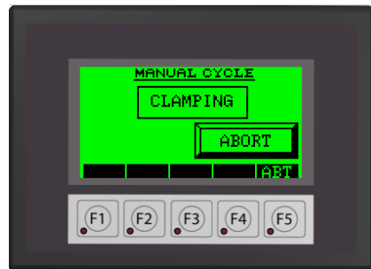
Figure 4-13, Manual Cycle, Clamping in Progress
