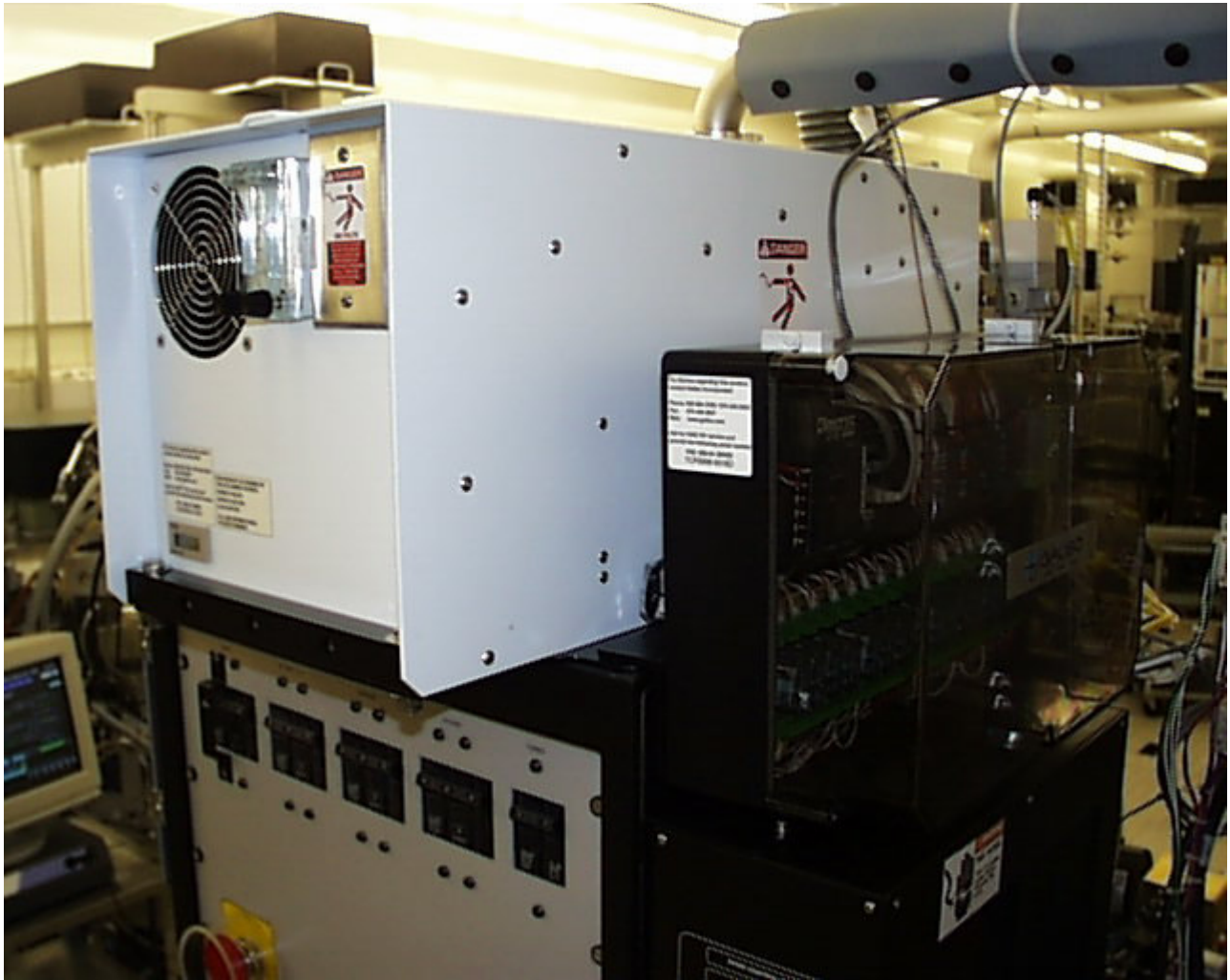
Galiso PLC shown mounted next to HGS unit.
